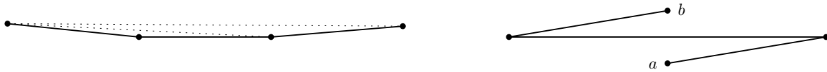
Figure 16: A path with unit length edges, that requires an edge of length 3 - \varepsilon for 2-edge-connectivity augmentation (left). A path between a and b where the stretch factor is large, but cannot be improved with additional edges (right).
